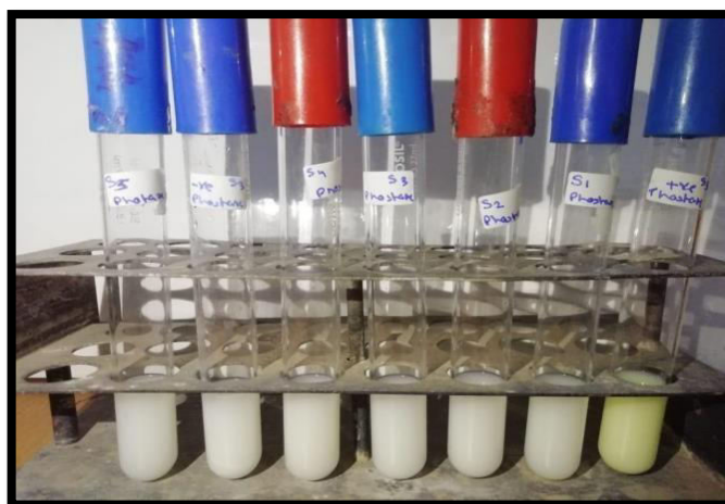
Fig.3: Phosphatase test results for samples 1 to 5
