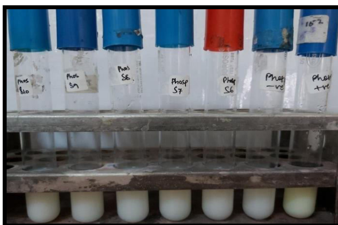
Fig.6: Phosphatase test results for samples 6 to 10
